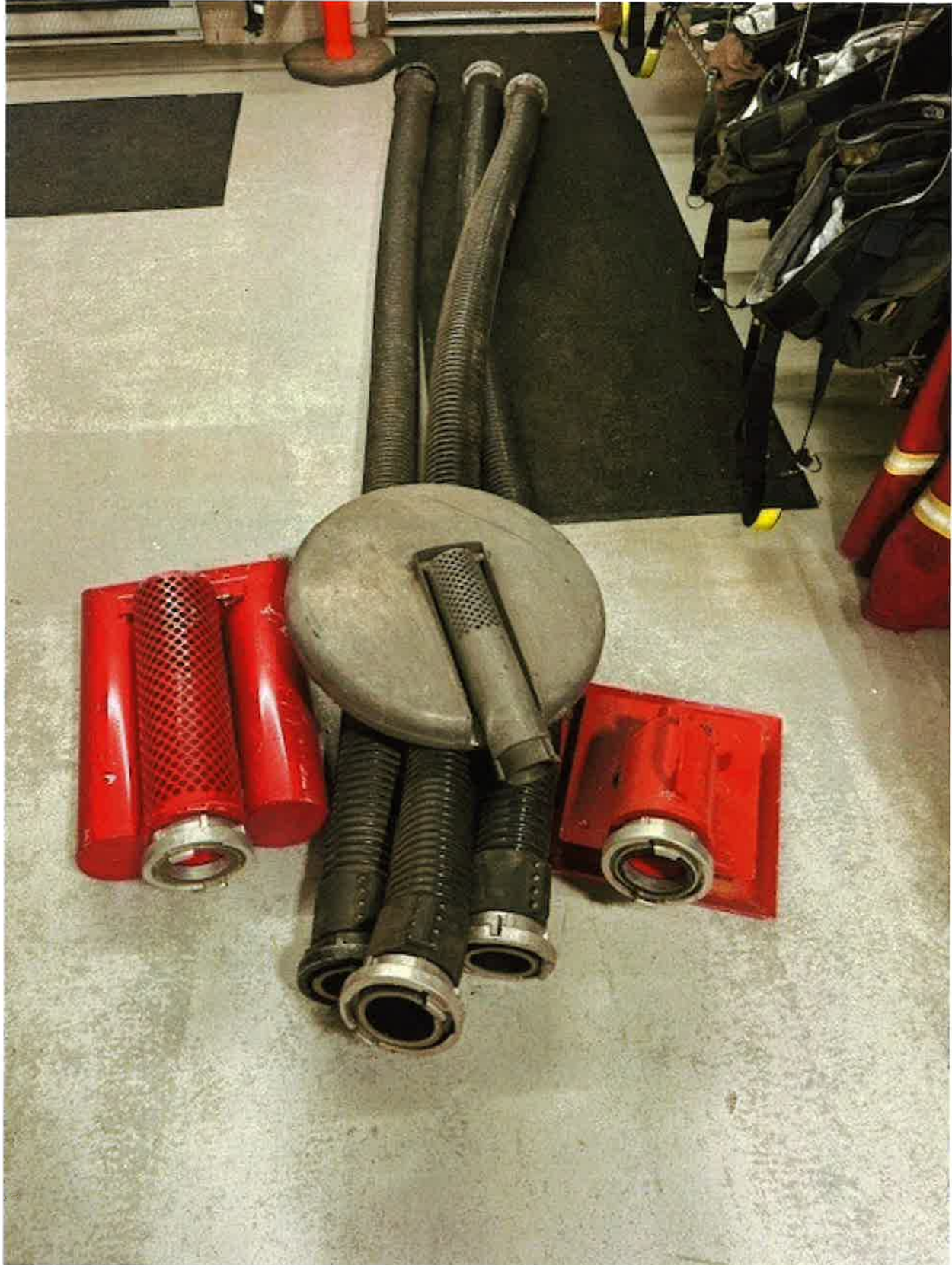
4-4"-10 Foot Storzs Hard Suction Pipes with 3 Suction Strainers (1 not in picture)
